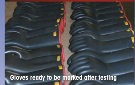
Glove electrical testing
